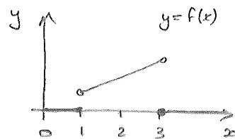
$$\begin{aligned} P(\text{resistance} < 2) &= \int_1^2 f(x) dx \\ &= \int_1^2 \frac{1}{4}x \cdot dx \\ &= \left[ \frac{1}{8}x^2 \right]_1^2 \\ &= \frac{1}{8}(2^2 - 1^2) \\ &= \frac{1}{8}(4 - 1) \\ &= \underline{\underline{\frac{3}{8}}}. \end{aligned}$$
